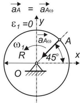
$$\vec{a}_A = \vec{a}_{A\varepsilon} + \vec{a}_{A\omega} = 0 \cdot \vec{T} + a_{A\omega} \vec{N} = R \cdot \omega_1^2 \vec{N}$$
